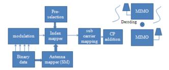
Fig. 1: MIMOI M Block Diagram
