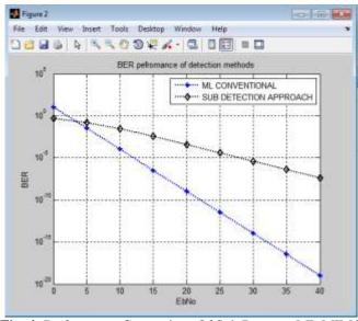
Fig. 4: Performance Comparison Of Sub Detector ML MIMO
